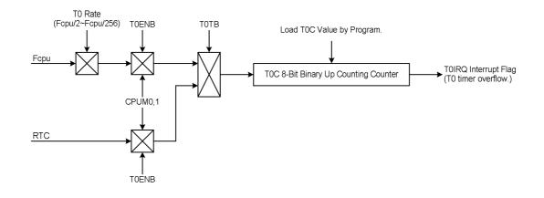
Note: In RTC mode, the T0 interval time is fixed at 0.5 sec and T0C is 256 counts.
