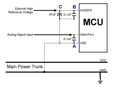
The analog signal is inputted to ADC input pin "AINn/P4.n" or "AINn/P0.n". The ADC input signal must be through a 0.1uF capacitor "A". The 0.1uF capacitor is set between ADC input pin and VSS pin, and must be on the side of the ADC input pin as possible. Don't connect the capacitor's ground pin to ground plain directly, and must be through VSS pin. The capacitor can reduce the power noise effective coupled with the analog signal.
