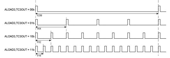
The PWM output pin is shared with GPIO and switch to output PWM signal as PWM3OUT=1 automatically. If PWM3OUT bit is cleared to disable PWM, the output pin exchanges to last GPIO mode automatically. It easily to implement carry signal on/off operation, not to control TC3ENB bit.
