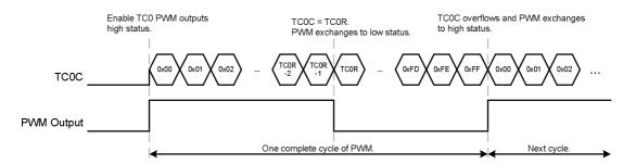
The PWM builds in four programmable resolution (1/256, 4/64, 4/32, 4/16) controlled by ALOAD0 and TC0OUT bits as PWM0OUT = 1.
