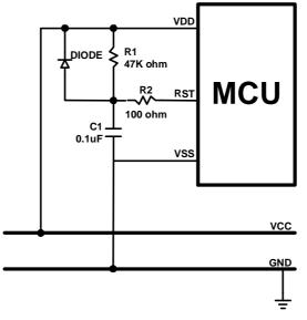
This is the better reset circuit. The R1 and C1 circuit operation is like the simply reset circuit to make a power on signal. The reset circuit has a simply protection against unusual power. The diode offers a power positive path to conduct higher power to VDD. It is can make reset pin voltage level to synchronize with VDD voltage. The structure can improve slight brown out reset condition.
