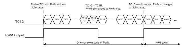
The PWM builds in four programmable resolution (1/256, 4/64, 4/32, 4/16) controlled by ALOAD1 and TC1OUT bits as PWM1OUT = 1. TC1R controls the high pulse width of PWM for PWM's duty. When TC1C = TC1R, PWM output exchanges to low status.
