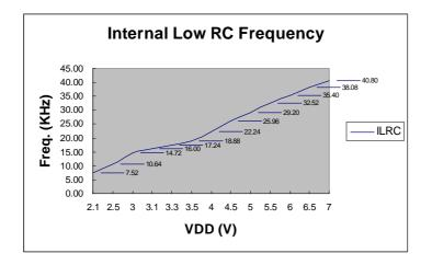
The internal low RC supports watchdog clock source and system slow mode controlled by "CLKMD" bit of OSCM register.
