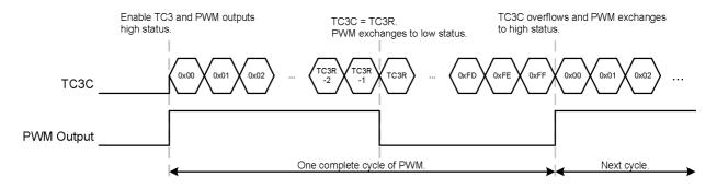
The PWM builds in four programmable resolution (1/256, 4/64, 4/32, 4/16) controlled by ALOAD3 and TC3OUT bits as PWM3OUT = 1. TC3R controls the high pulse width of PWM for PWM's duty. When TC3C = TC3R, PWM output exchanges to low status.
