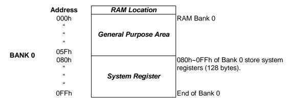
The 96-byte general purpose RAM is in Bank 0. Sonix provides "Bank 0" type instructions (e.g. b0mov, b0add, b0bts1, b0bset...) to control Bank 0 RAM in non-zero RAM bank condition directly.
