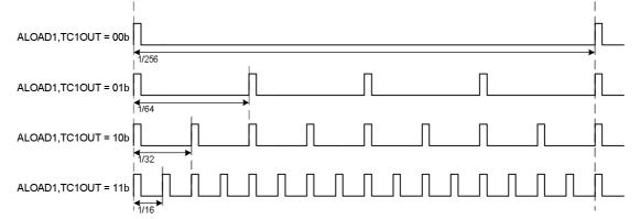
The PWM output pin is shared with GPIO and switch to output PWM signal as PWM1OUT=1 automatically. If PWM1OUT bit is cleared to disable PWM, the output pin exchanges to last GPIO mode automatically. It easily to implement carry signal on/off operation, not to control TC1ENB bit.
