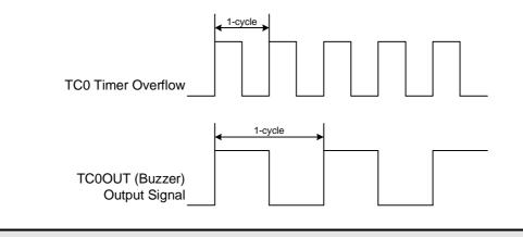
• Note: Buzzer output is enabled, and "PWM0OUT" must be "0".
