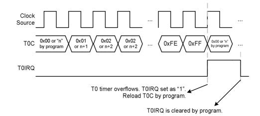
T0 clock source is Fcpu (instruction cycle) through T0rate[2:0] pre-scaler to decide Fcpu/2~Fcpu/256. T0 length is 8-bit (256 steps), and the one count period is each cycle of input clock.
