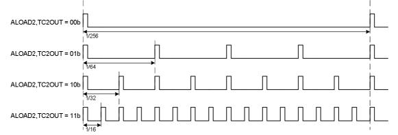
The PWM output pin is shared with GPIO and switch to output PWM signal as PWM2OUT=1 automatically. If PWM2OUT bit is cleared to disable PWM, the output pin exchanges to last GPIO mode automatically. It easily to implement carry signal on/off operation, not to control TC2ENB bit.
