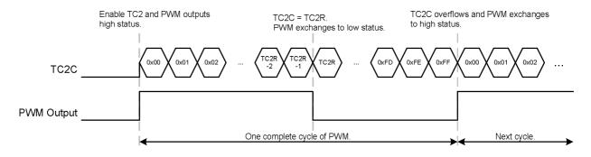
The PWM builds in four programmable resolution (1/256, 4/64, 4/32, 4/16) controlled by ALOAD2 and TC2OUT bits as PWM2OUT = 1. TC2R controls the high pulse width of PWM for PWM's duty. When TC2C = TC2R, PWM output exchanges to low status.
