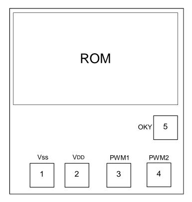
Note: The IC substrate must be connected to GND.
