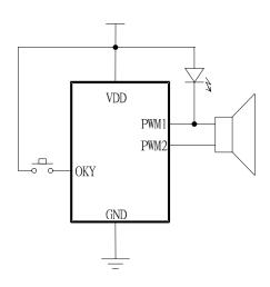
While driving motor, one capacitor is suggested to put between VDD and GND.
